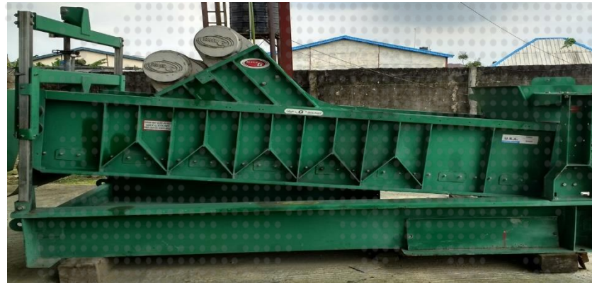
Hi-G Dryer fitted with Super G vibrator Motors
